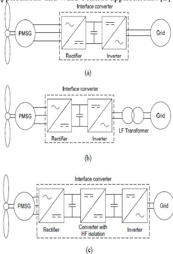
**Fig 1:** Block diagram of interfacing converters
