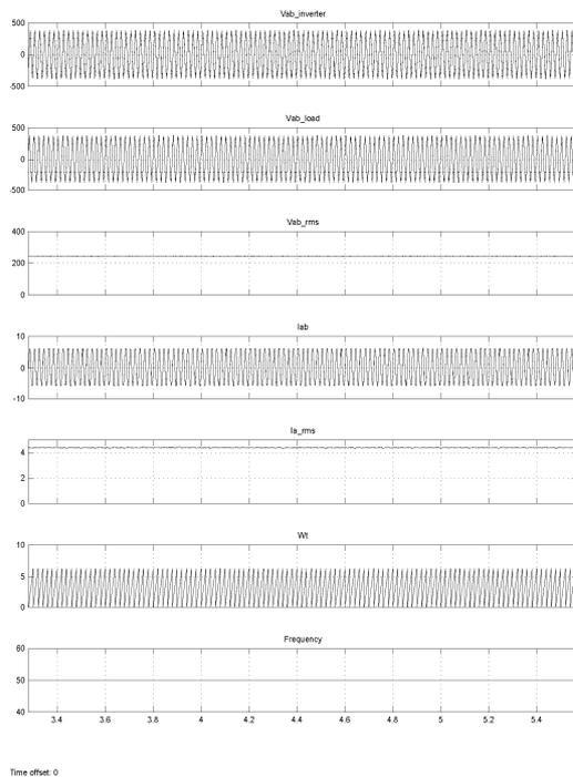
**Fig 6:** Load voltage and current RMS values
