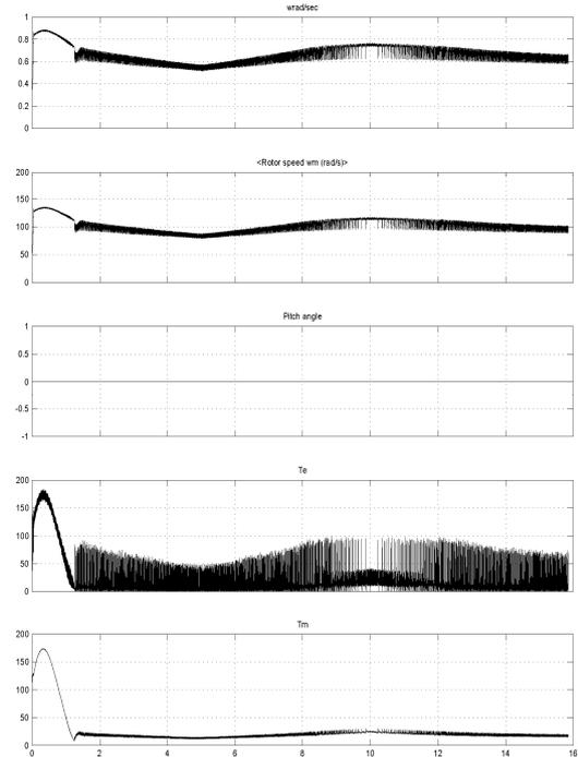
**Fig 4:** Mechanical, Electrical Torque and rotor speed with pitch angle
