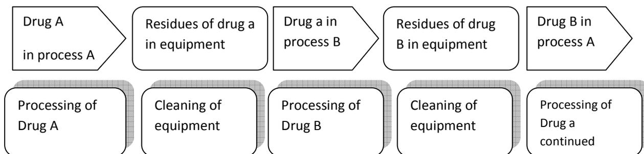
**Figure 1: Carry-over for Common Equipment**
