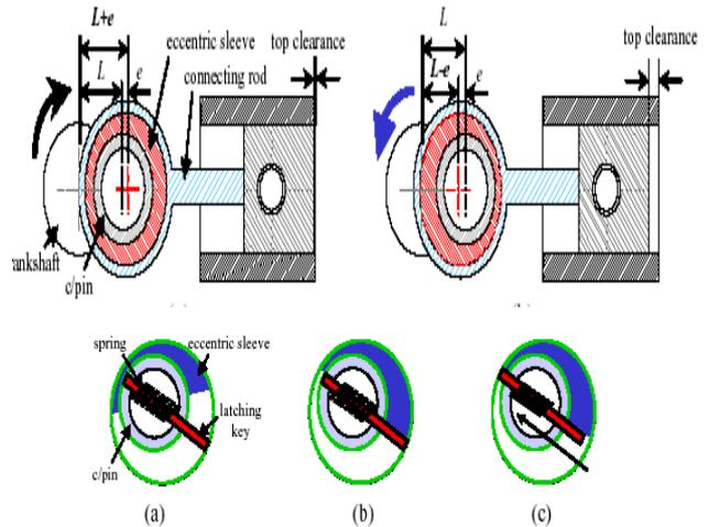
**Fig.6 latching system of capacity modulation of compressor**
