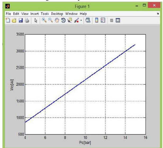
**Fig.4. Compressor Power & Condenser Pressure**
