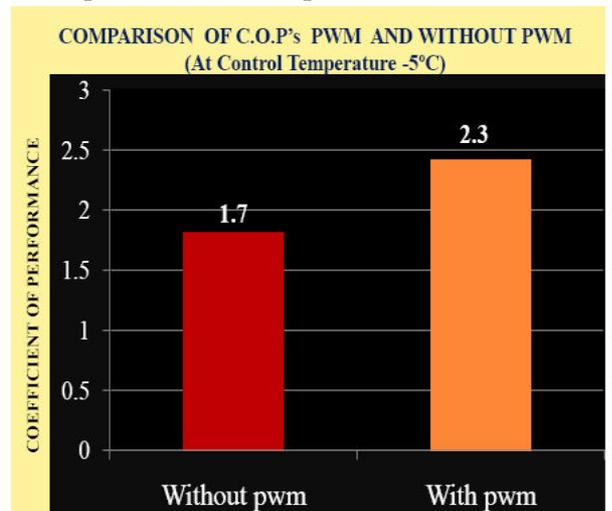
6. Comparison of coefficient of performance with and without pulse width modulation technique at control temperature -25°C.
