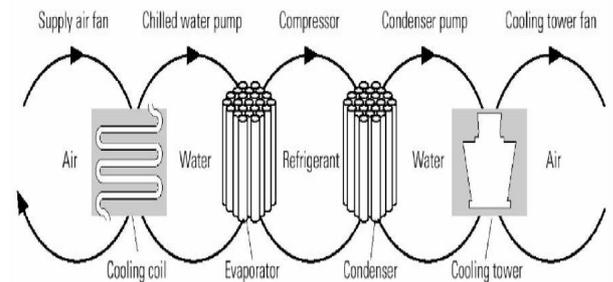
**Fig.3. Heat Transfer Loop in Refrigeration System**
