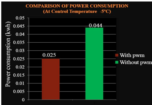
3. Comparison of power consumption with and without pulse width modulation technique at control temperature -25°C.
