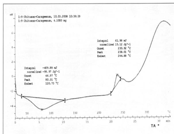
The DSC thermogram of interacted sample of carrageenan with chitosan was shown in figure 5. The interacted sample of carrageenan and chitosan had shown an endothermic transition at 81.29°C with a heat content of (-) 99.97 J/g. The heat content of the system from (-) 554.90 J/g, it was in case of carrageenan (-) 212. 90 J/g and in case of chitosan was decreased to (-) 99.97 J/g. The decrease in the heat content might be due to interaction of carrageenan and chitosan.
