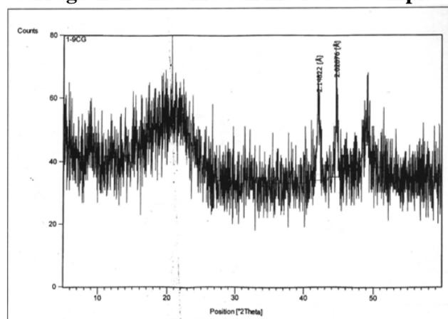
The x-ray diffraction pattern has shown the diffused pattern indicating the amorphous nature of the polymers. To confirm the structural changes due to interaction of carrageenan and chitosan, the x-ray diffraction pattern of the interacted sample was recorded and it was shown in figure 4. It has also shown the diffused pattern indicating the interacted polymer sample was present in the amorphous state.
