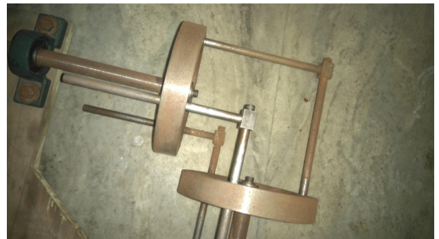
Fig 2: Working of gearless power transmission
