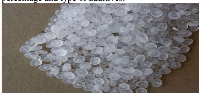
Fig 3.1: Polypropylene M110 (CIPET Raipur)
