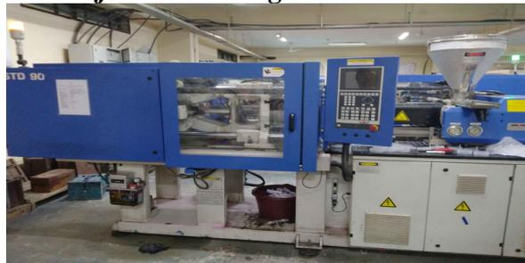
Fig 1: Plastic injection molding machine (CIPET Raipur)
