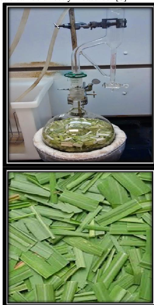
Fig. 1:- Clevenger Extraction Apparatus & Plant material
