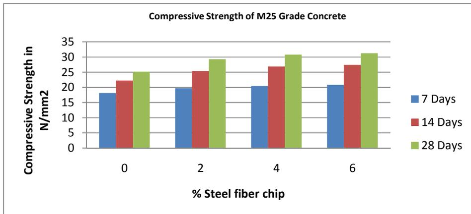
**Graph 1 – Compressive Strength of M25 Grade Concrete**
