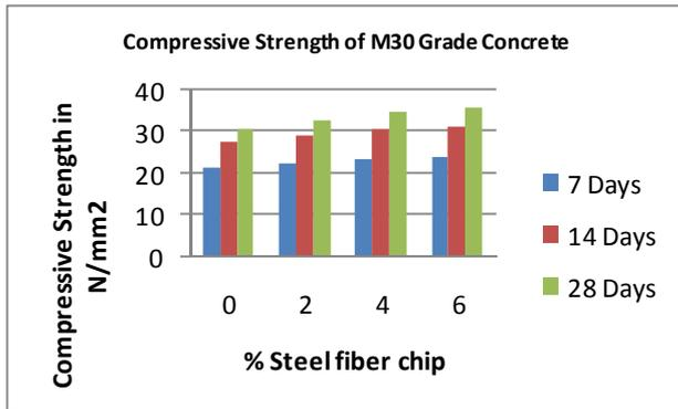
**Graph 2 – Compressive Strength of M30 Grade Concrete**
